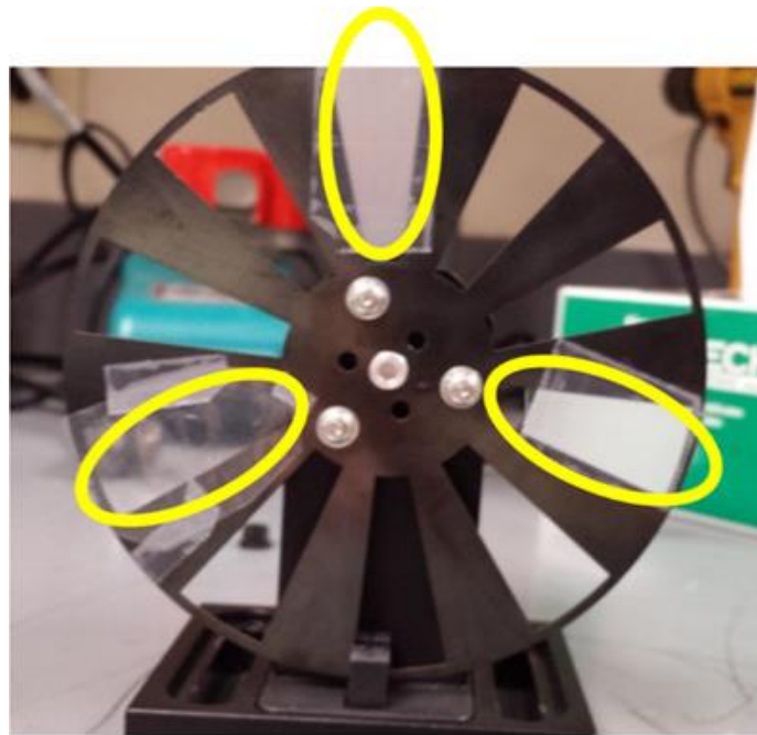
Figure 23: Optical chopper used for beam modulation in the temporal response studies, with three windows covered with various layers of polymer sheet to simulate absorption (highlighted in yellow).
