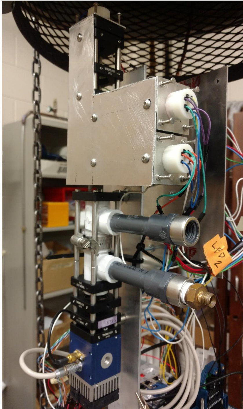
Figure 16: Overall lab sensor. From top to bottom: LEDs and pitch optics, PVC flow cell, focusing lenses, detector.
