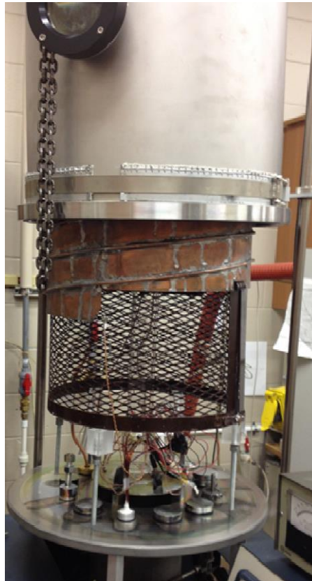
Figure 19: UCF environmental chamber. The outer chamber comes down to hold a vacuum (down to ~2Torr) while the copper shroud is wrapped in copper tubing for the flow of liquid nitrogen (LN 2 ) to cool the system to low temperatures.
