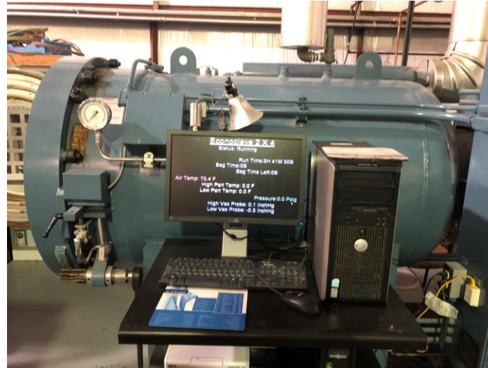
Autoclave Curing Stage
