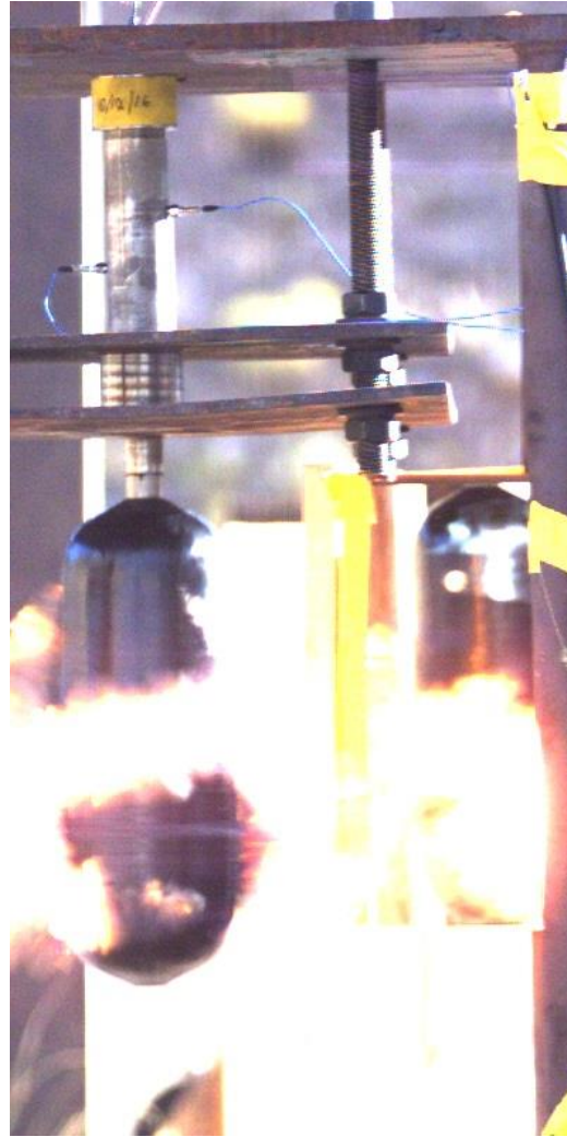
Secondary fractures after single opening
