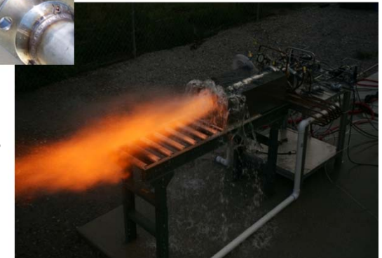
ATK/Plasma process test with eductor attached to workhorse engine
