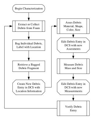
Figure 3: Debris Fragment DCS Workflow
