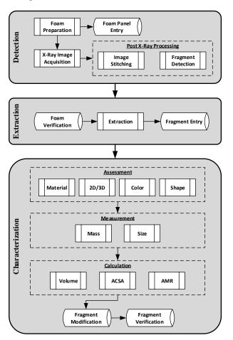
Figure 2: Post-Impact Phase Workflow
