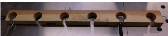
Figure 4 Wooden fixture for placement of sensors.
