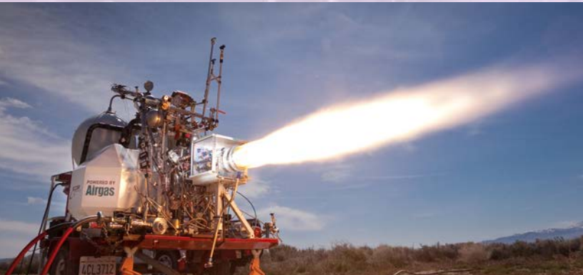
October 2012: Test firing of XCOR Aerospace's liquid oxygen/kerosene engine destined to power the company's Lynx suborbital reusable vehicle.
